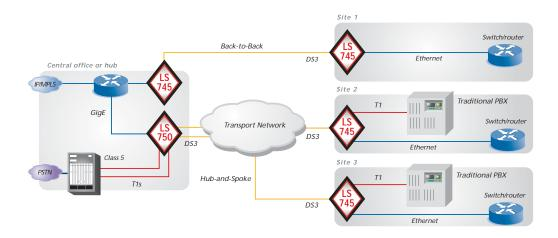
The LoopStar 745 and LoopStar 745P deliver cost-effective Ethernet and/or T1 services over DS3.
